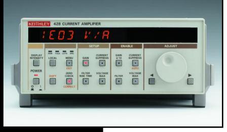
The Model 428-PROG Programmable Current Amplifier converts fast, small currents to a voltage, which can be easily digitized or displayed by an oscilloscope, waveform analyzer, or data acquisition system. It uses a sophisticated "feedback current" circuit to achieve both fast rise times and sub-picoamp noise. The gain of the Model 428-PROG is adjustable in decade increments from  $10^{3}$ V/A to  $10^{11}$ V/A, with selectable rise times from  $2\mu$ s to 300ms.
